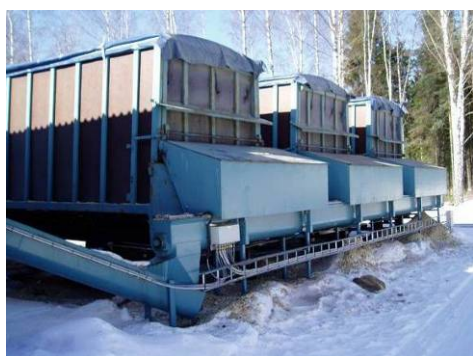
Containerrack for flis (foto: SWECO Grøner AS)
