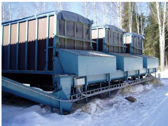
Containerrack for flis (foto: SWECO Grøner AS)
